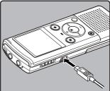
3 Make sure that the recorder is stopped, and then connect the USB cable to the connecting port on this recorder. Windows:
