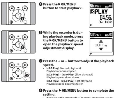
If you leave the recorder for 3 seconds, the setting will be applied and the recorder will return back to the original screen.
