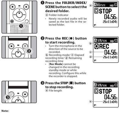
For VN-8100PC only If a recording is made in stereo modes ([192 kbps] or [128 kbps]), it will be a monaural recording through the built-in microphone, and the same audio will be recorded on both Left channel (Lch) and Right channel (Rch).
