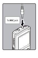
The external microphone and other devices can be connected and the sound can be recorded. Connect as follows by the device to be used.
